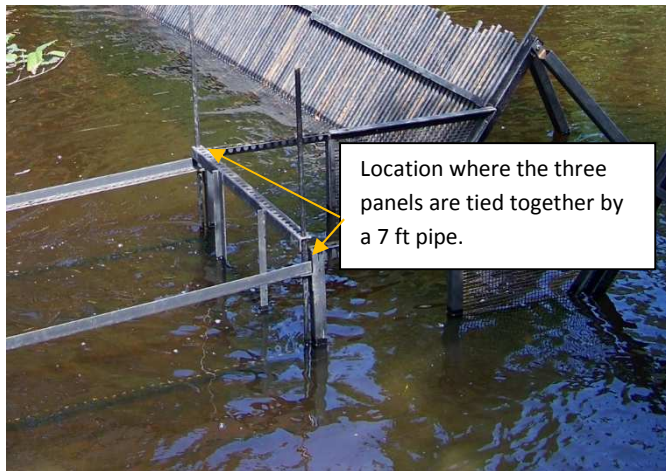
Figure 16. View of the entrance panels, front panel of the collection box and drilled angled steel, tied together by 7 ft pipes.
